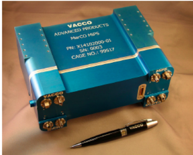
Figure 40: A VACCO cold gas system.
