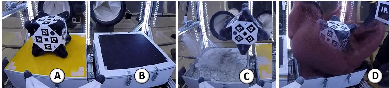
Figure 19: Test surfaces: (A) low-friction and (B) high-friction rigid surfaces, (C) crushable comet regolith simulant, and (D) granular, low-cohesion garnet sand.
