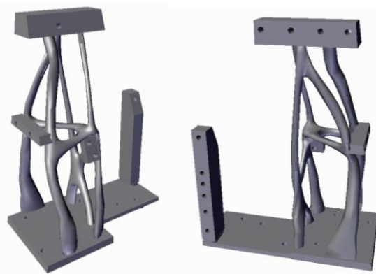
Fig. 20: Design of the third “Rusty Tower” bracket obtained by topology optimisation
