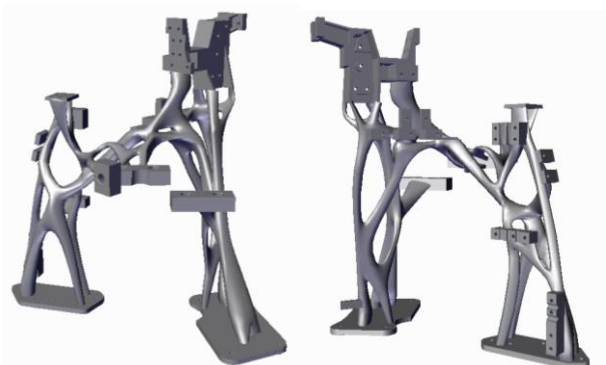
Fig. 18: Design of the first “Rusty Tower” bracket obtained by topology optimisation
