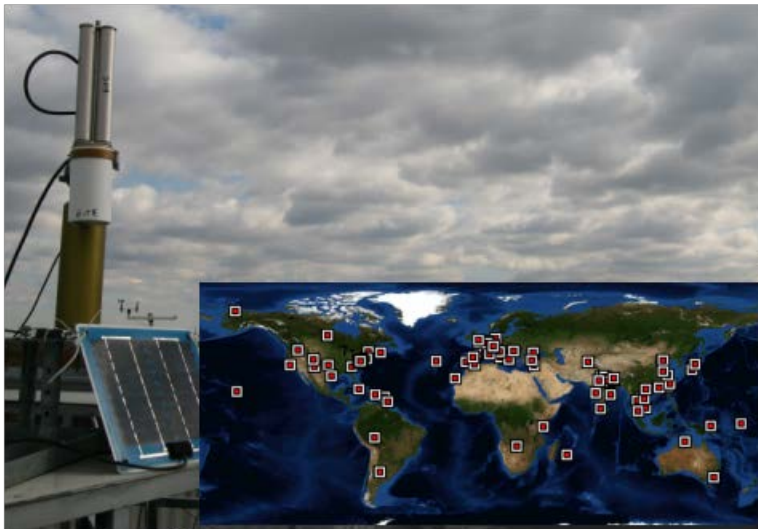
Figure 4-8. Zenith position of the CIMEL™ radiometer in cloud mode. Global distribution of the 271 AERONET stations used to retrieve cloud optical thickness is shown in the inset.
