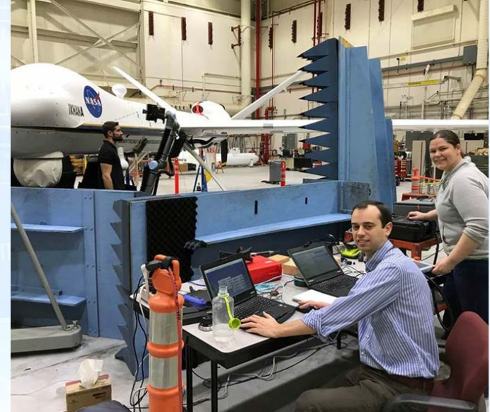
Collaborative robotic arm and laser tracker used to test antenna on UAS at AFRC
