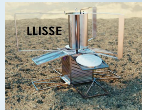
LLISSE-W probe with wind turbine for recharging the battery.
