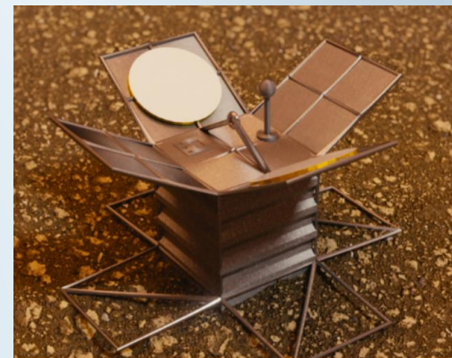
LLISSE-B probe powered only by charged battery.
