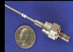
MEMS seismic event sensor Courtesy: Tom Pike
