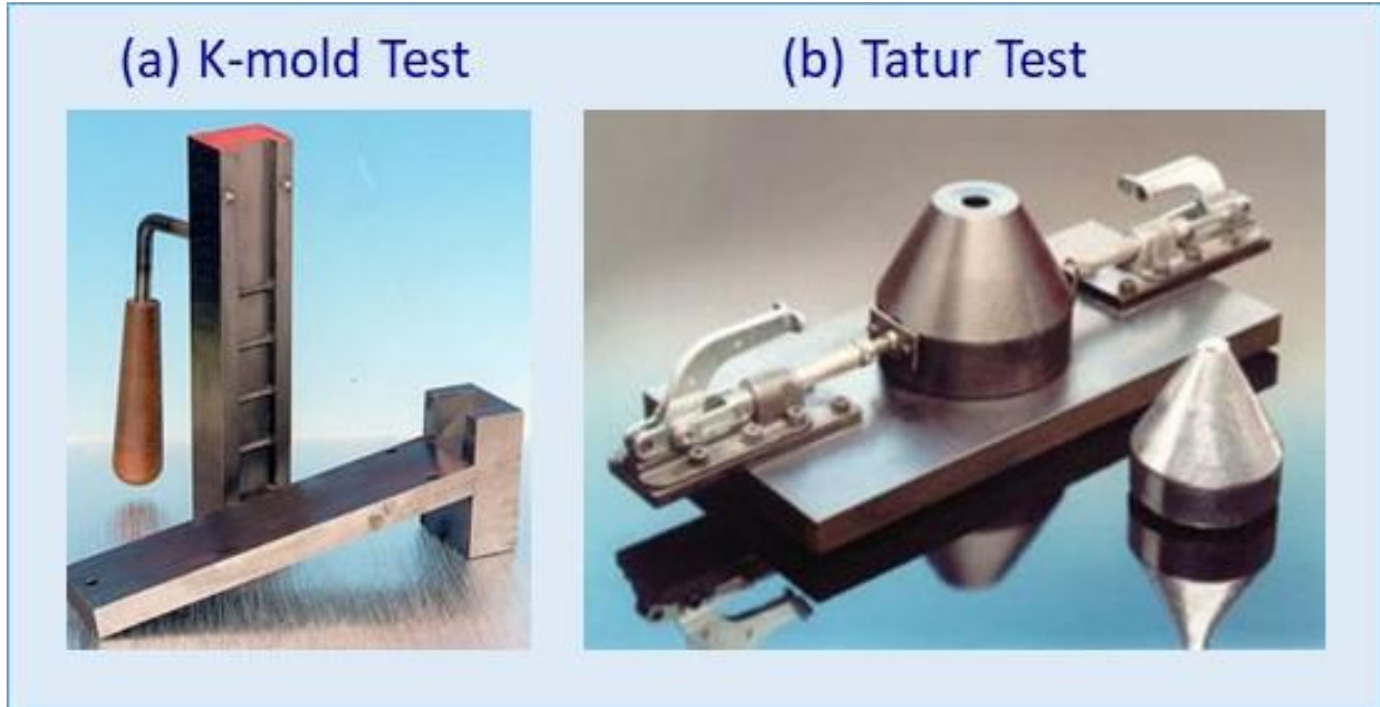
Figure 14. Design options for reference dies to determine the inclusion/porosity content for producing low-defect castings [ref. 22]: (a), the K-mold test; (b), the Tatur test. Note that the K-mold configuration is more adaptable to die casting operations.
