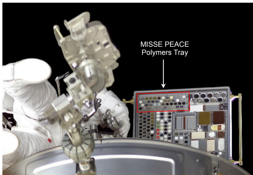
Figure 1. During a spacewalk on August 16, 2001, astronaut Patrick Forrester installs MISSE PEC 2 on the ISS Quest Airlock.
