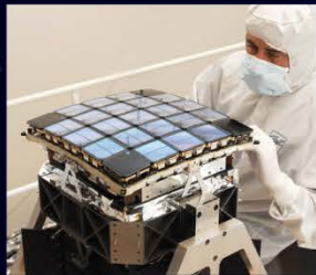
Focal Plane 95 Mega pixels, 42 CCDs
