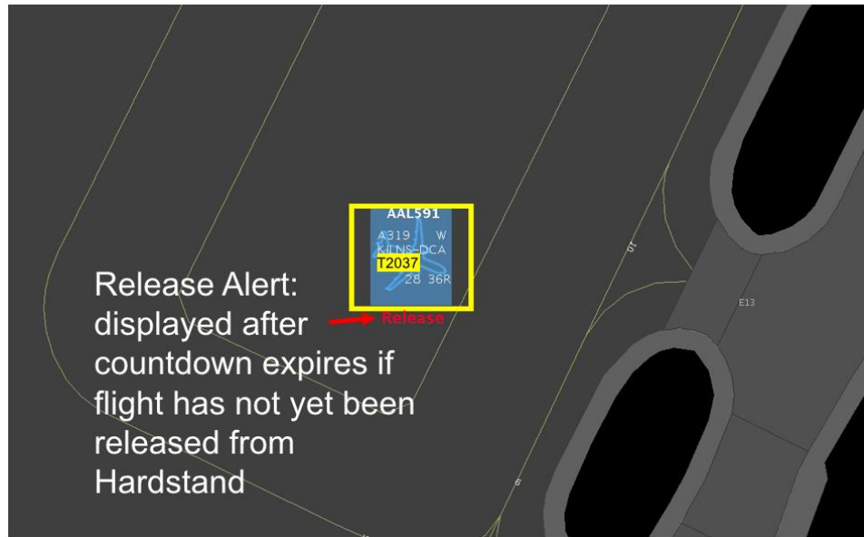
Figure 4.8. Alert to Release From Hardstand.
