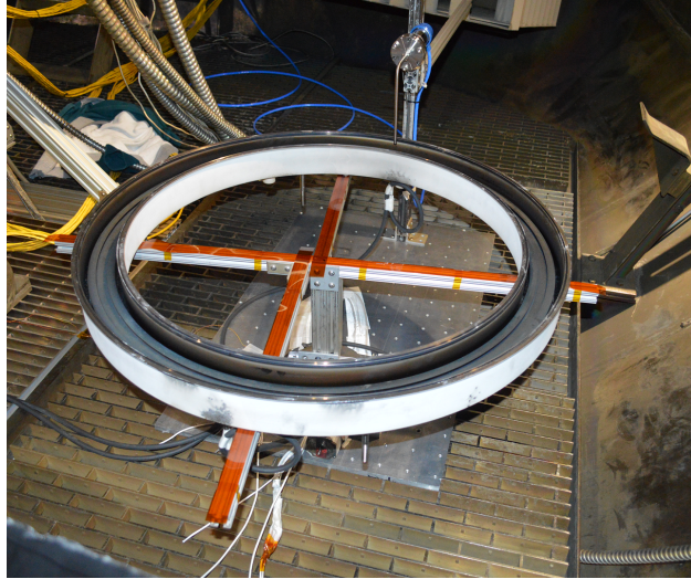
Figure 4.26: A photograph of the test setup, installed in the LVTF. Here, the outer channel is aligned and ready for testing. The Pitot tube and Stabil gauge can be seen in the background; the anode and rotational stage in the foreground; and the rigid aluminum plate connecting the two underneath.
