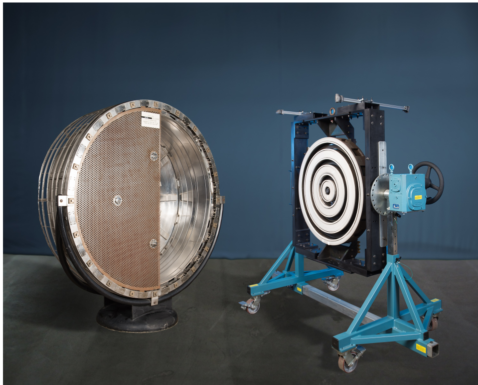
50 years of high-power electric propulsion at NASA Glenn Research Center: a 1.5-meter diameter mercury ion thruster tested to 200 kW in 1967 (which has since been modified into a display unit) on the left and the X3 NHT, which was tested to 102 kW in 2017, on the right. Image courtesy NASA.
