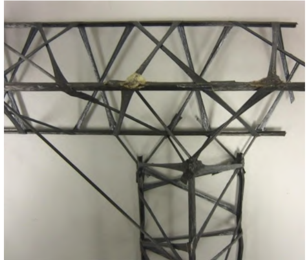
Figure 12. Spanner Joint Geometry. Joining trusses with a separation distance was accomplished using a heated iron to attach CF/PEEK rods from the nodes of one truss to the nodes of the other (spanner joint).
