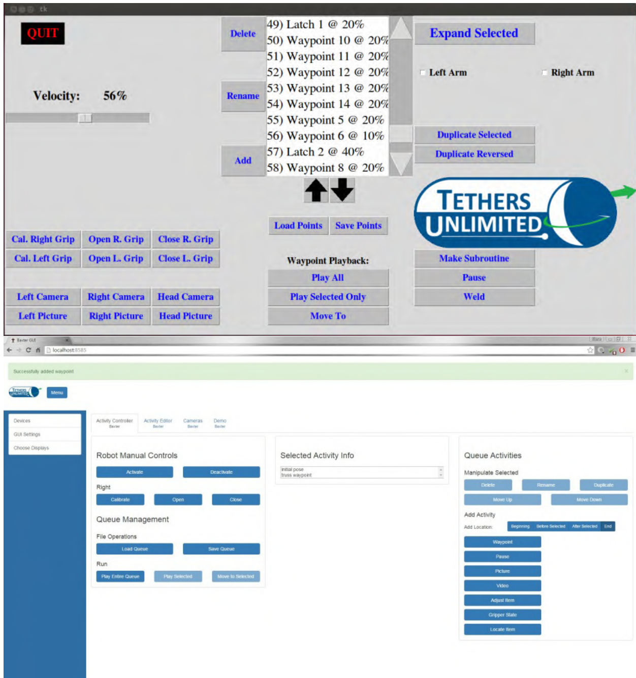
Figure 44. Example of running an application from two different GUI interfaces. The first GUI (top) was quickly built for initial testing using the Python TK library. We later upgraded to a custom HTML-based GUI (bottom) for a cleaner cross-platform interface with more sophisticated controls.
