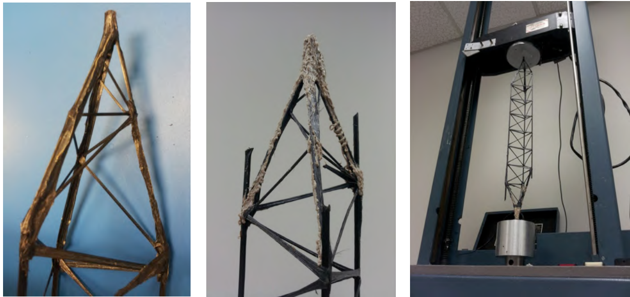
Figure 14. Point Joint Geometry Fabrication and Testing. Using SpiderFab techniques, we formed pointed tips on the ends of a truss (left), reinforced them with PEEK resin (center), and performed compression to evaluate their structural integrity (right).
