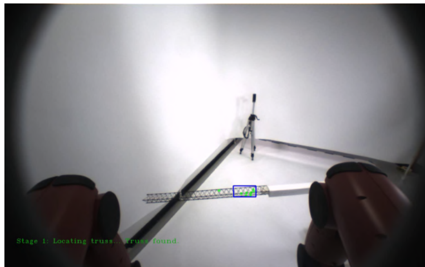
Figure 50. Truss location approximation using homography algorithms.
