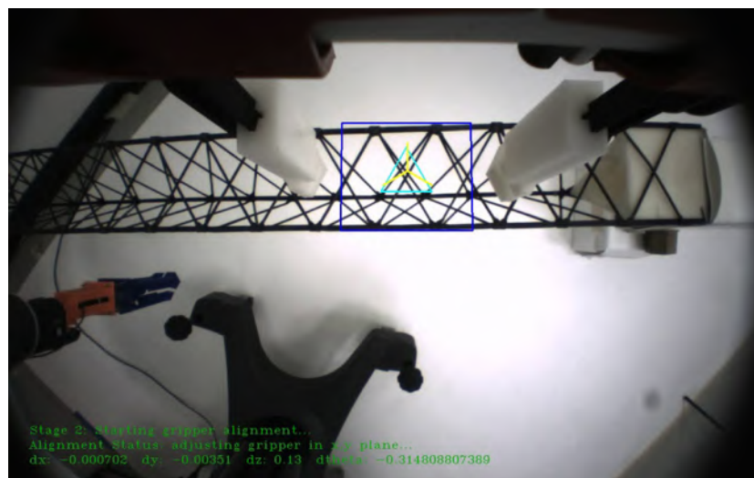
Figure 52. Robot identifying truss grasping point.
