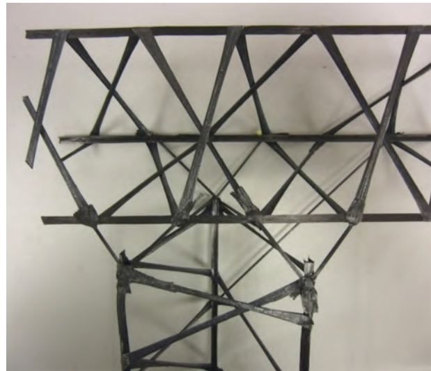
Figure 58. Spanner Joint Geometry. Highly efficient joints can be formed between truss elements using the Joiner Spinneret to add additional CF/PEEK ligaments between nodes on the truss..
