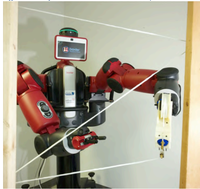
Figure 24. Test of pultrusion of long elements using the SpiderFab spinneret as an end-effector on the Baxter robot.
