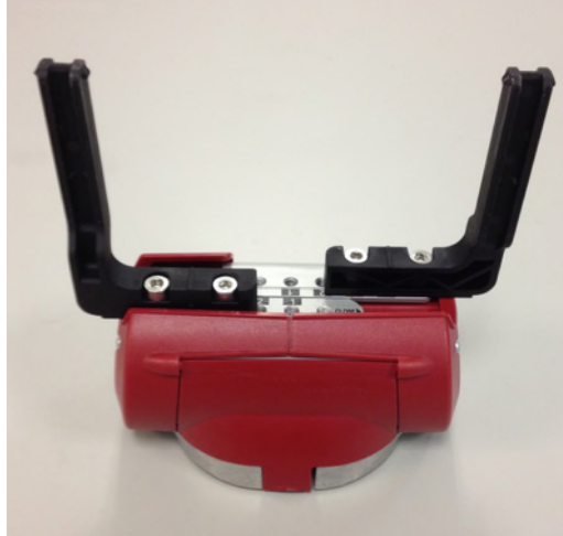
Figure 46. An unmodified Rethink Robotics parallel gripper designed for use with the Baxter robot.
