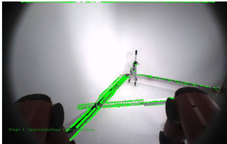
Figure 49. Truss identification using edge and feature detection algorithms.
