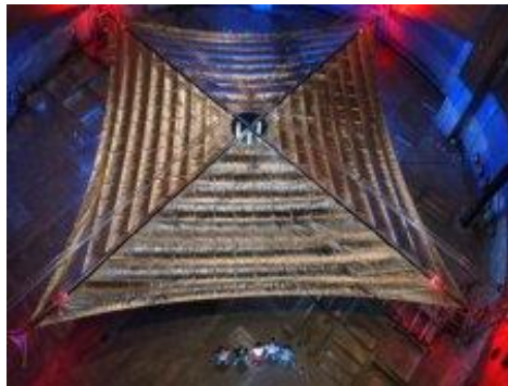
Figure 18: An image of the 34m x 34m Sunjammer sail.
