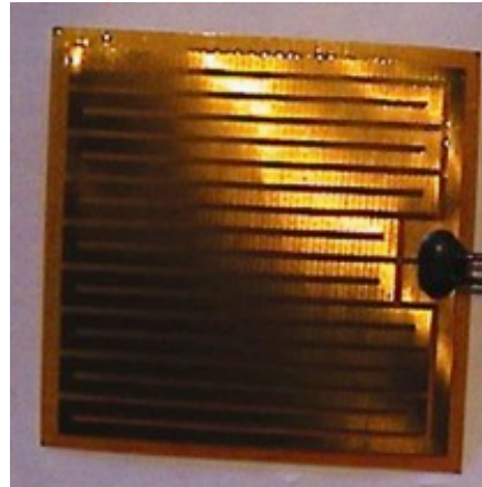
Figure 4.27—DuPont Kapton Strip Heater.
