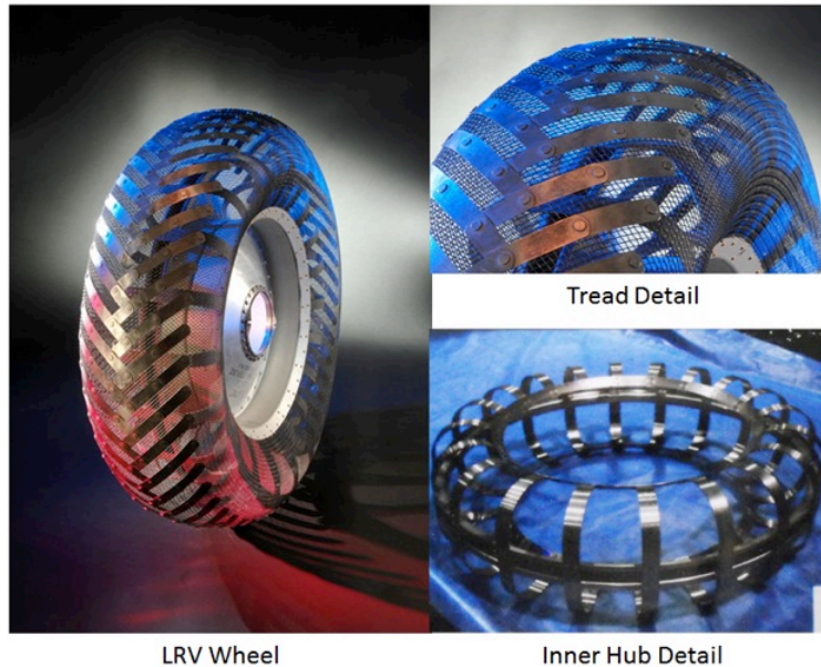
Figure 4.6—Lunar rover wheel.
