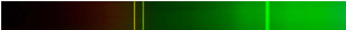
Fig. 34 Hg lines of 579.066, 576.960 and 546.074 nm as seen through HOE 1 and recorded with a CMOS camera, Kodak Z812 IS.
