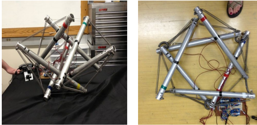
Figure 44: Tensegrity under Star Elongation Method of Collapse.
