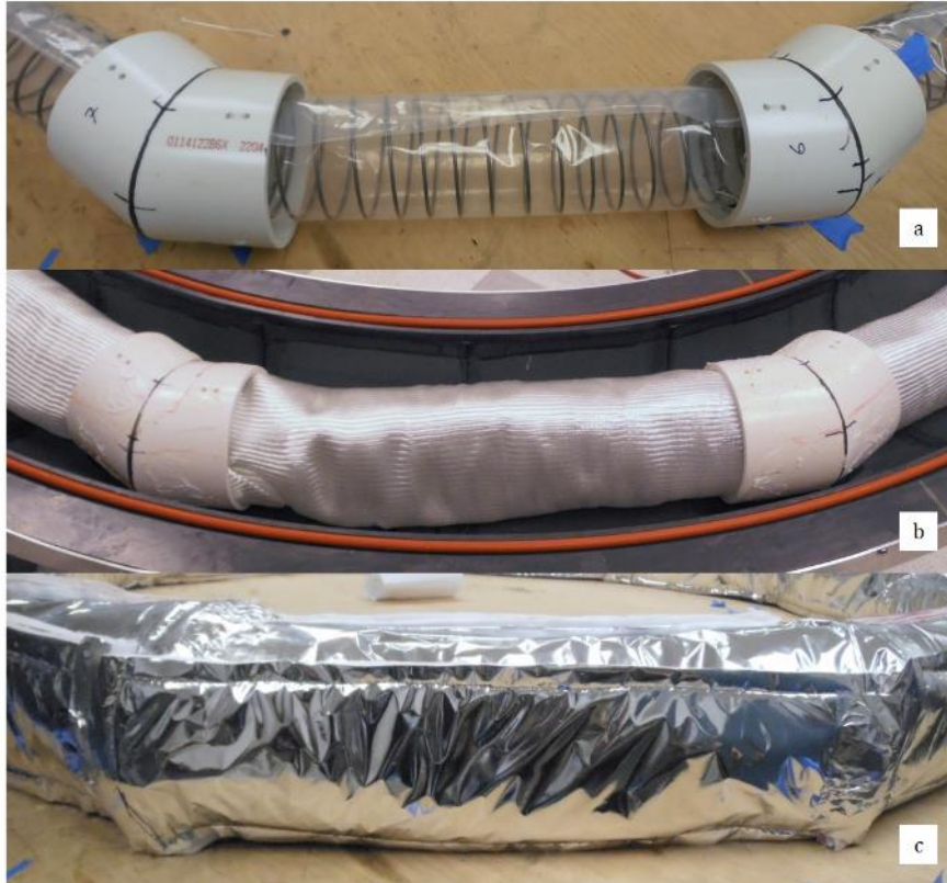
Figure 3.11 Close-up of toroidal enclosure segment with a) inner core, b) fiberglass sleeve over core, c) thermal blanket
