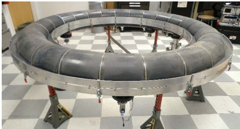
Figure 3.18 Vacuum chamber used for thermal testing
