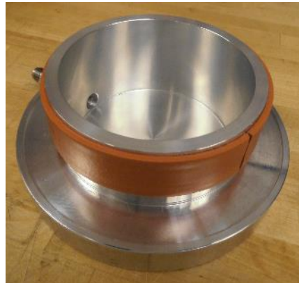
Figure 3.16 Vapor containment end caps and closed cell foam
