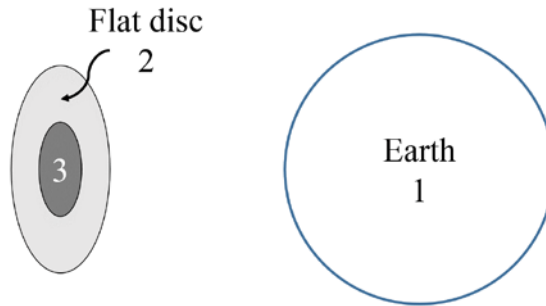
Figure 3.6 View factor numbering designation where surface 1 is a sphere, surface 2 is a flat disc (not including surface 3 as a hole)
