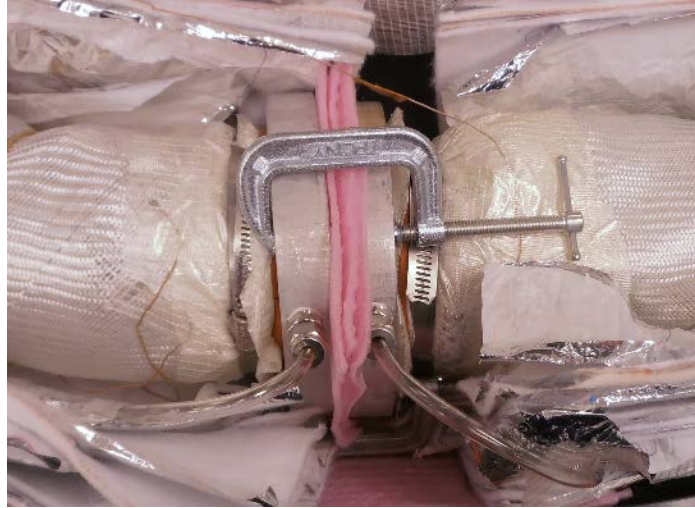
Figure 3.17 End caps with ends of plastic and fiberglass secured
