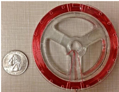
Figure 12: Copper coil as used in both Separate and Unfold deployment tests
