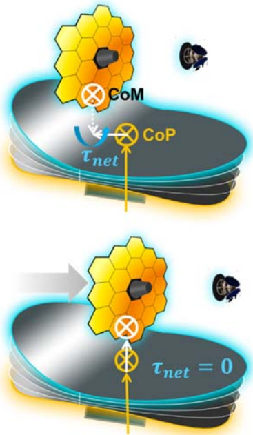
Fig. XIII: Reducing the center of pressure-center of mass offset of a cryogenic telescope at L2
