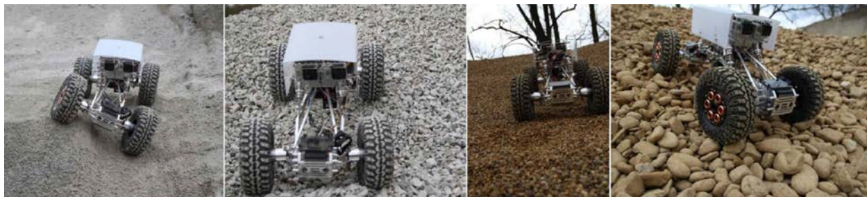
Figure 143: Rock Crawler mobility platform ascending and descending piles of different material types (pea gravel, 1-inch limestone, pea river rock, 3-inch river rock).
