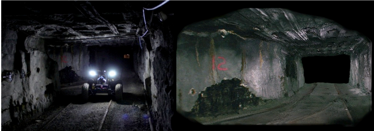
Figure 43: A mapping robot explores a terrestrial underground space using active illumination (left). An immersive virtual model of the environment is created using camera and LIDAR fusion techniques (right).
