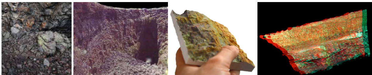
Figure 4: Research conducted extensive field testing and explored existing and new methods for visualization of robot data, including mesh models (left), point rendering (center left), 3D printing (center right), and anaglyph stereo (right).
