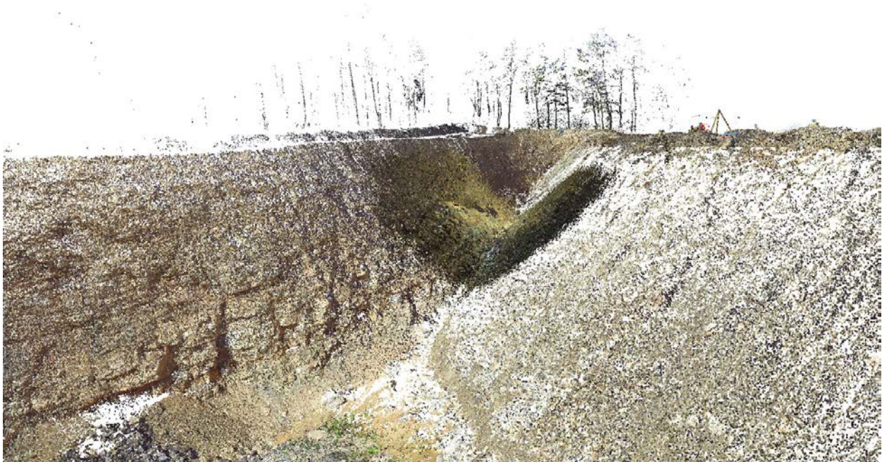
Figure 94: Fourth of four robot scans (saturated section) overlaid with FARO ground truth measurements
