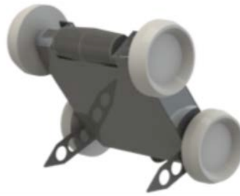
Figure 22: Cavehopper robot ready to execute a hop (left). Cavehopper leaping into a pit
