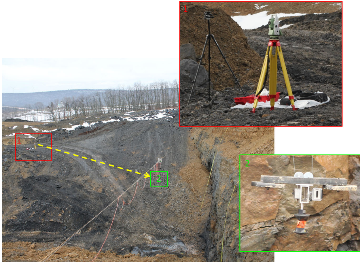
Figure 81: The skylight wall-modeling payload was surveyed with an automated total station. The total station provided valuable data on the stability of the Tyrolean system for sensing and ground truth locations for modeling viewpoints. This configuration also illustrates a possible 2-robot scenario for modeling the skylight. A survey robot on the rim could provide line-of-sight tracking for the SkyCam modeler to greatly increase accuracy over internal-only sensing.
