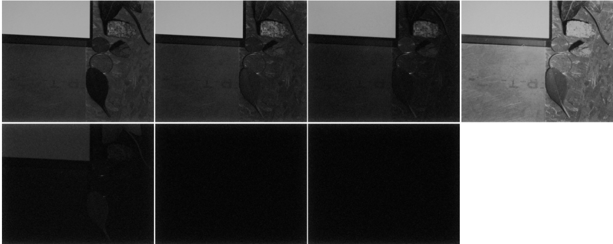
Figure 39: The same scene illuminated by an LED array light source. The light source illuminates the scene effectively in the visible range (400-700 nm), but as the filters progress farther into the NIR range, the images go black.
