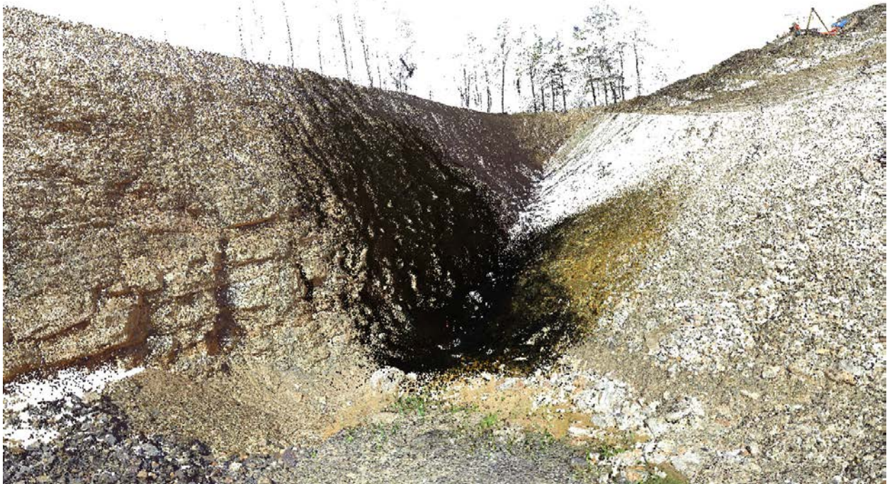
Figure 92: Second of four robot scans (saturated section) overlaid with FARO ground truth measurements
