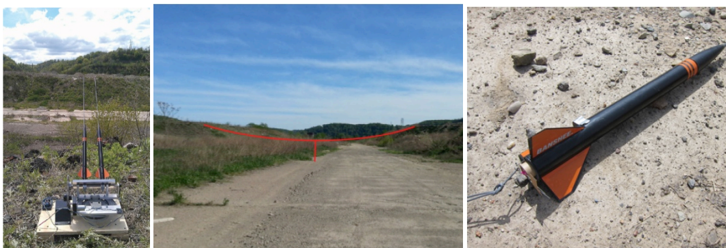
Figure 140: Rocket launch platform for tether deployment (left). This system might be mounted to a lander that is positioned near the edge of the skylight. Tests in earth gravity and atmospheric demonstrated deployed cable distance of 34m (center) with a hobby rocket; efficiency and distance only improve on the Moon. A fishing line tether is attached to the rocket that is used to pull the Tyrolean cable across (right).
