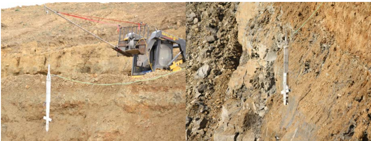
Figure 28: Experimental Setup for Cable-Descent Modeling. A skid-loader and boom rigging were utilized to suspend the device over the skylight wall (left). Ferret borehole sensor scans the wall face while free-hanging (right). A green tether is utilized for data communications.
