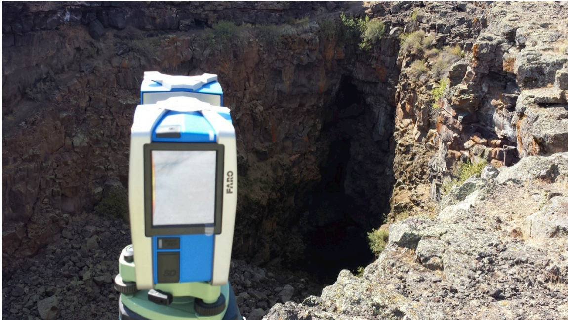
Figure 159: FARO instrument used for ground truth data collection at the edge of King's Bowl pit.
