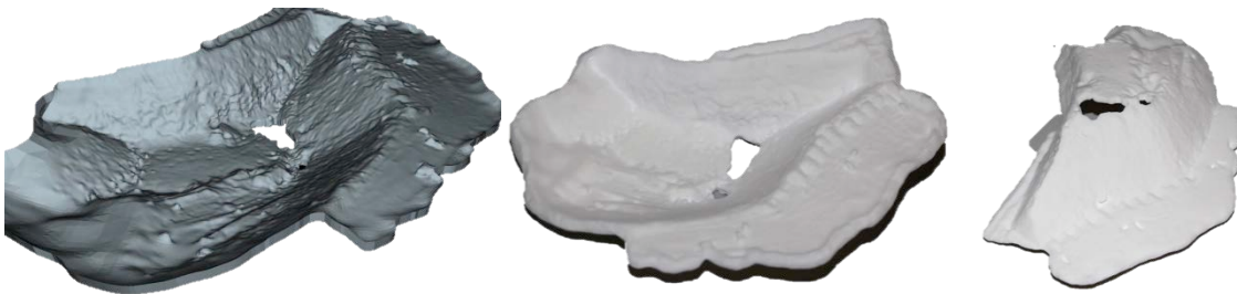
Figure 125: Computer rendering of mine pit 3D model created by robots (left). Top view of 3D printed shell model looking into the pit (center) and reverse view (right).
