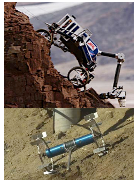
Figure 25: Cliffbot descending a rocky slope (top). Axel rover descending a slope, viewed from the tether anchor point (bottom). [Images credit: NASA/JPL]
