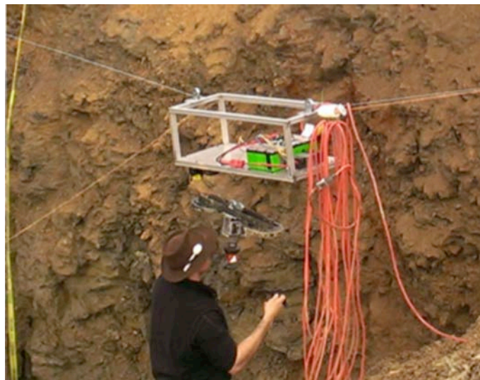
Figure 129: The first Tyrobot prototype included motorized raise-lower for a payload, but Tyrolean traverse was done manually, by pulling on cables from the pit rim. Command of the raise-lower mechanism happened through a wire (orange cable in image) strung along the Tyrolean line.
