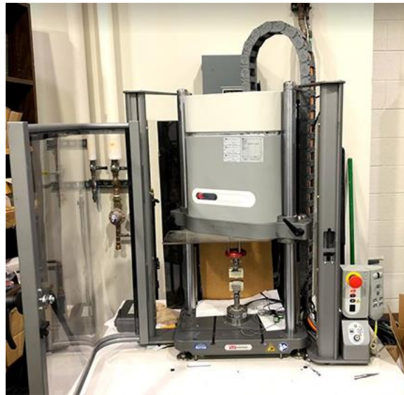
Figure 1: Instron ElectroPuls E1000 used to determine flexure strength of asteroid regolith simulant.
