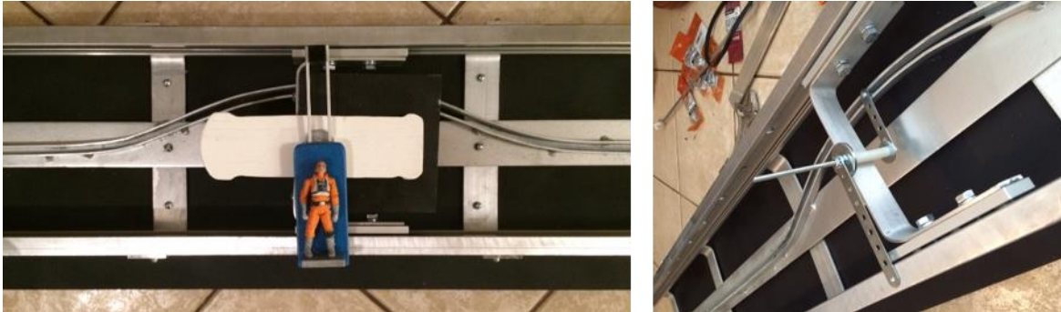
Figure 15: 1/20th scale model of the guide track actuation approach
