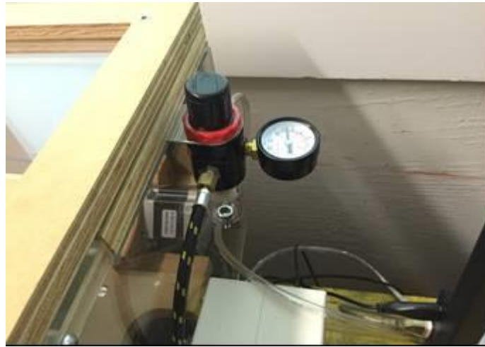
Figure: Spray pressure is regulated and adjustable
