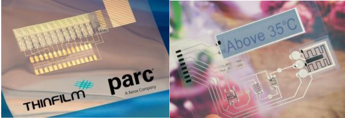
Figure 31 Xerox PARC and ThinFilm addressable memory and its application in a temperature sensing tag.
