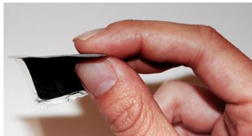
Figure 36 Imprint Energy ZincPoly™ printed rechargeable battery
