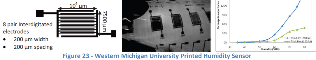
Figure 23 - Western Michigan University Printed Humidity Sensor
