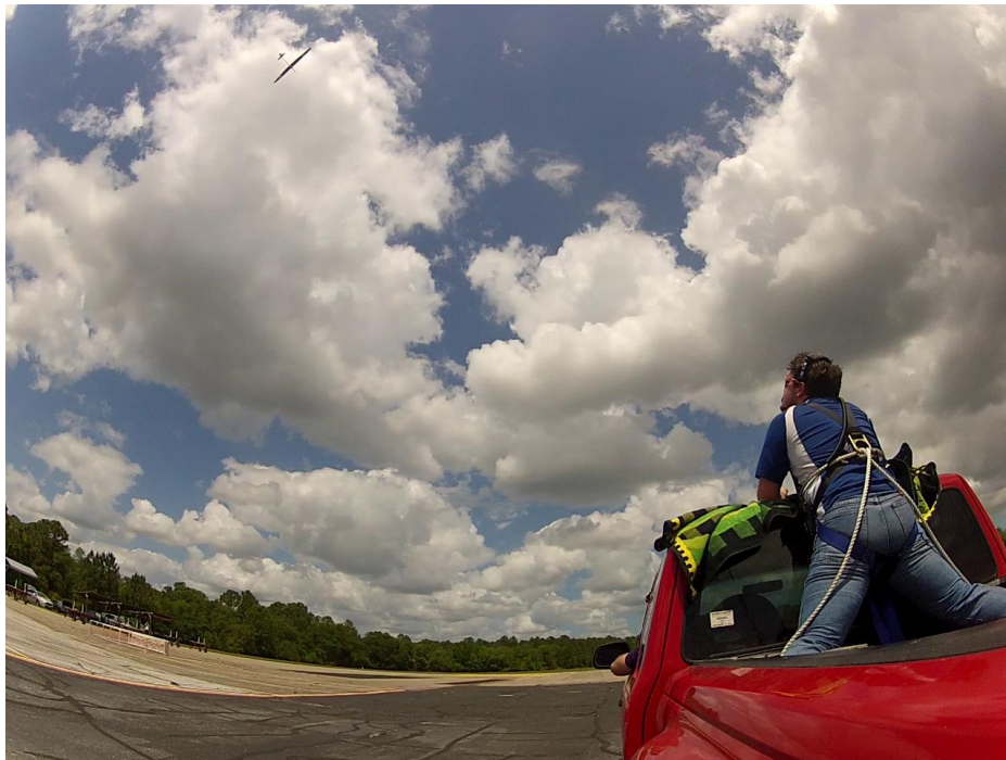
Figure 32. Manual control flight testing at Deland R/C field along runway from behind pilot (aircraft is connected via nylon line)
