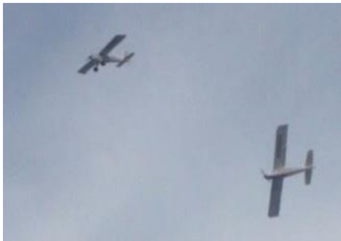
Figure 6. Two R/C Timbers connected by a nylon cable while attempting to hold line tension
