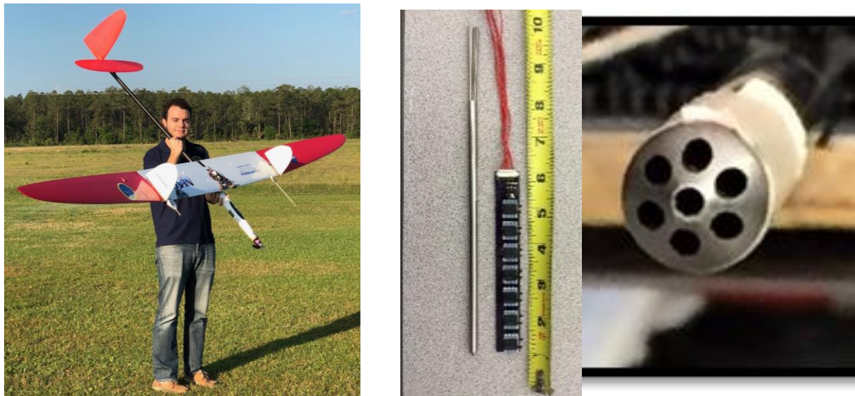
Figure 16. Prototype aircraft with pitot probe and 7-hole air data probe on opposite wings (left); 7-hole probe and pressure transducers (center) and front view of 7-hole probe (right)
