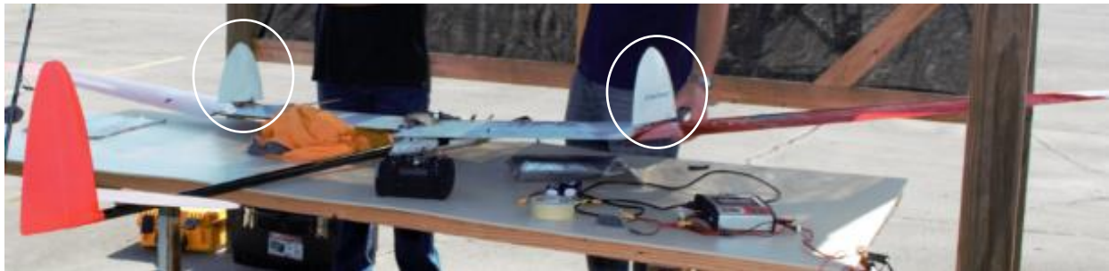
Figure 22. Prototype aircraft with double lateron configuration (surfaces identified by white circles).
