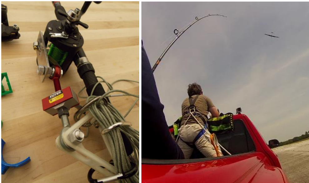
Figure 14. “Fishing Reel Mechanism” with Futek load cell (left); Fishing pole/line in use during flight test in which pilot controls aircraft (right)
