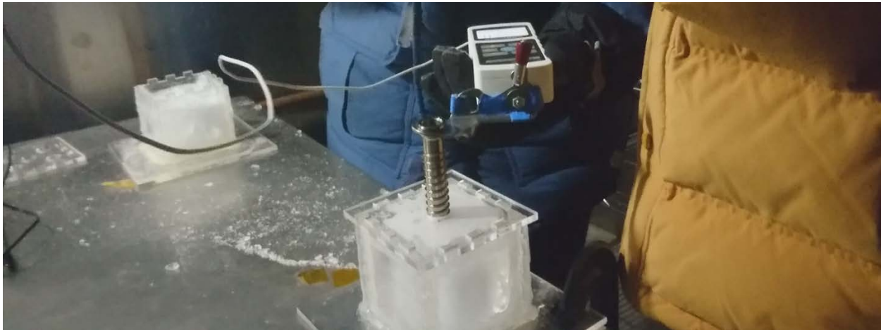
Figure 30 Experiment to measure the energy required to insert and remove an ice screw
