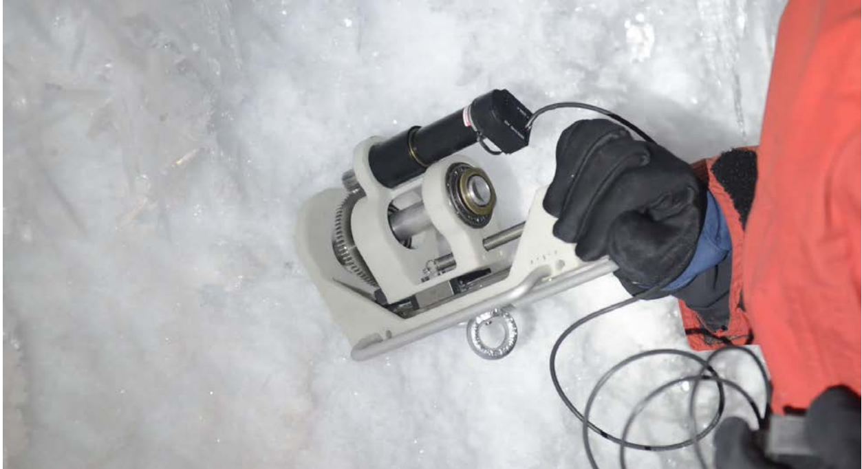
Figure 70. The ISEE did not anchor well in low density hoarfrost ice.
