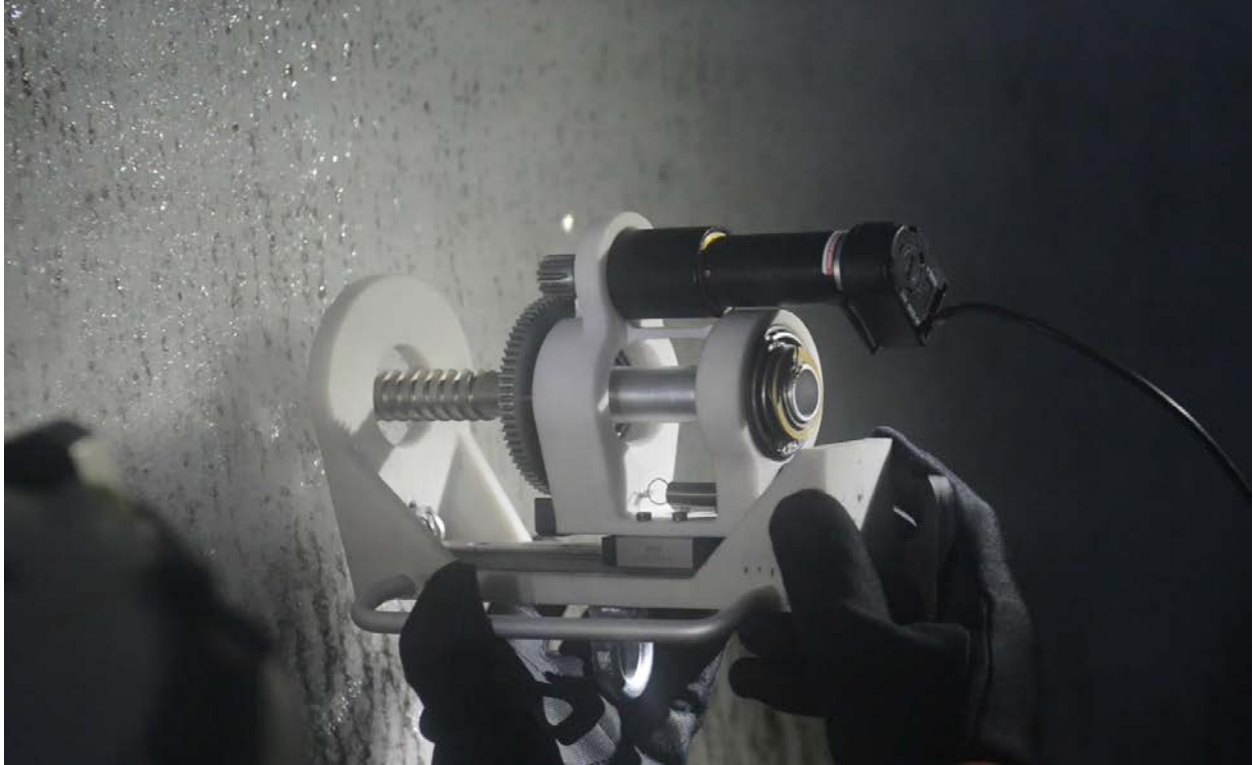
Figure 69. ISEE preload test in Helo Cave, a fumarolic ice cave on Erebus volcano in Antarctica.
