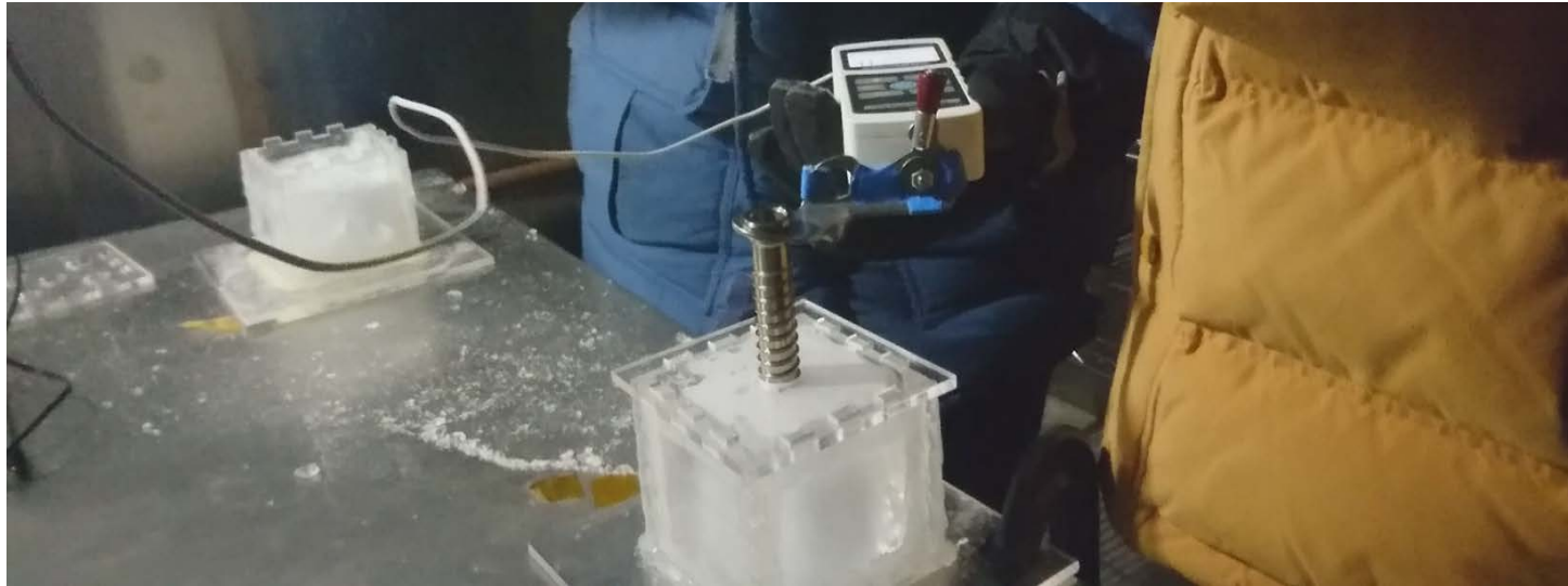
Figure 49 – The maximum torque measured during the insertion of the ice screw was 3.619 Nm. In order to get this number, the force gauge measured the perpendicular force to the ice screw at a distance of 72 mm from the center of the ice screw. If this maximum torque is assumed to be the torque required during the entire insertion of the screw, it would require about 341.2 J of energy.
