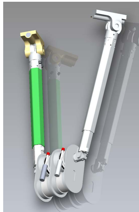
Figure 4 Prototype design of DM's front/rear section with two limbs
