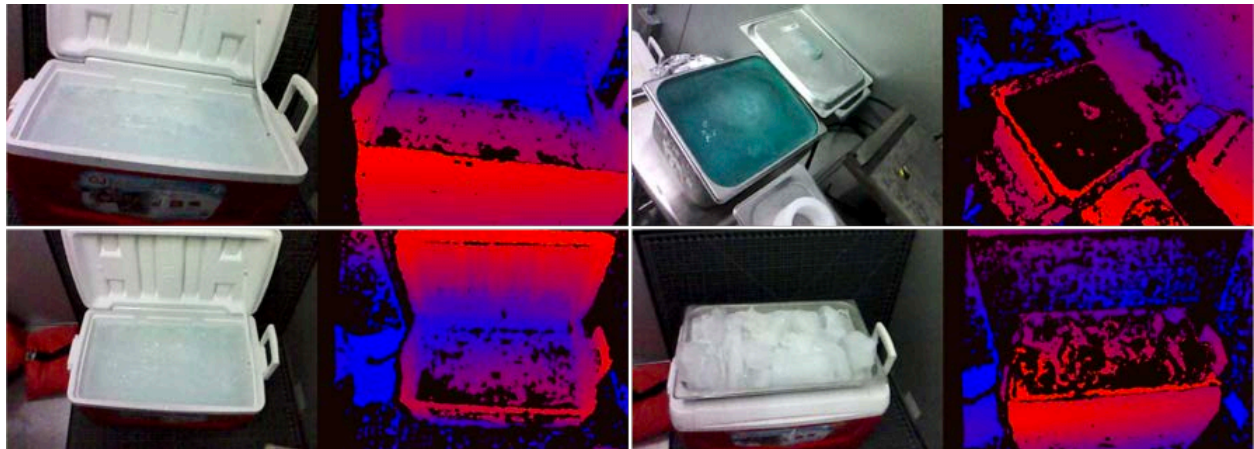
Figure 37: Assisted stereo on ice. Sensor: Intel infrared structured-light sensor. Material: artificial ice at JPL. The top-right image shows that the sensor does not work on translucent ice. The other images show convincing results for opaque ice.
