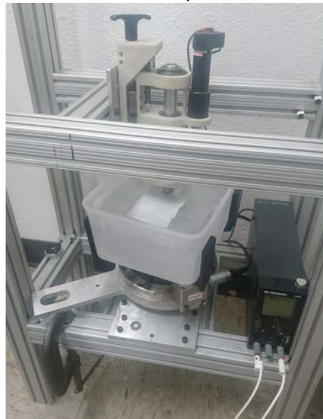
Figure 71. Ice screw end effector force / torque testbed, with ISEE mounted and ATI Gamma sensor beneath the ice block. The insulating sheet shown is placed beneath the screw before the experiment is initiated.
