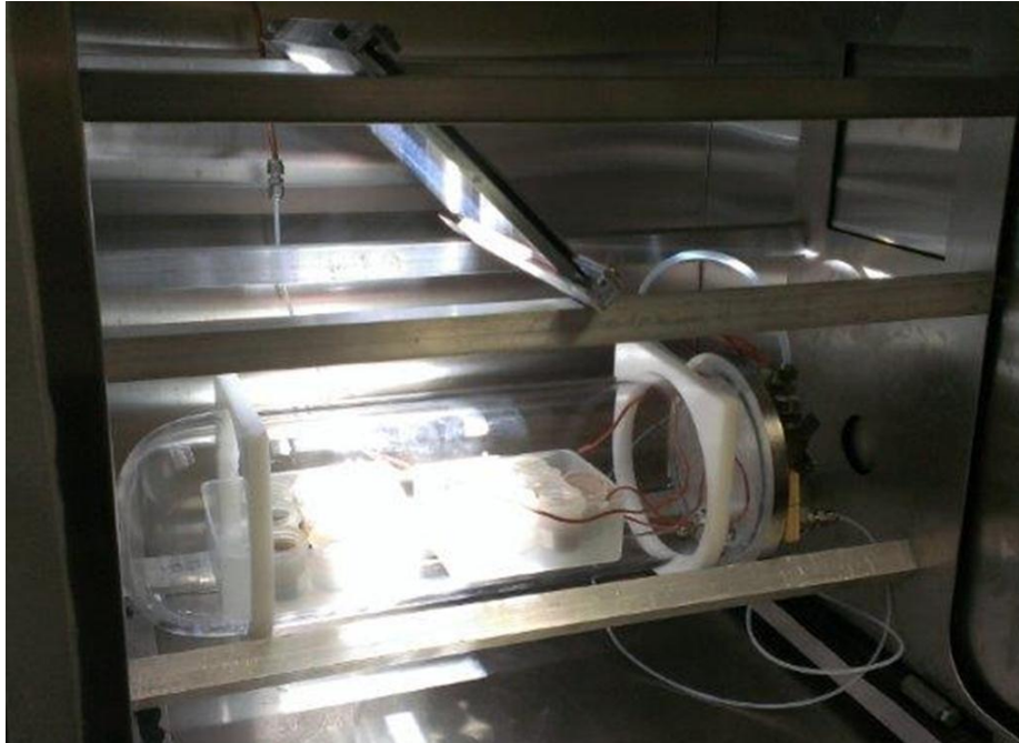
Figure 2. Interior of the Mars simulator environmental cabinet showing reflecting mirror, quartz chamber, sample tray, eighteen samples with twelve of them in direct illumination and six of them in shade, thermistor leads for temperature measurement in and out of regolith, end plate for pressure and electrical access, and cradle to hold quartz-tube Mars chamber. This configuration was used in an uninterrupted five-week simulation campaign.
