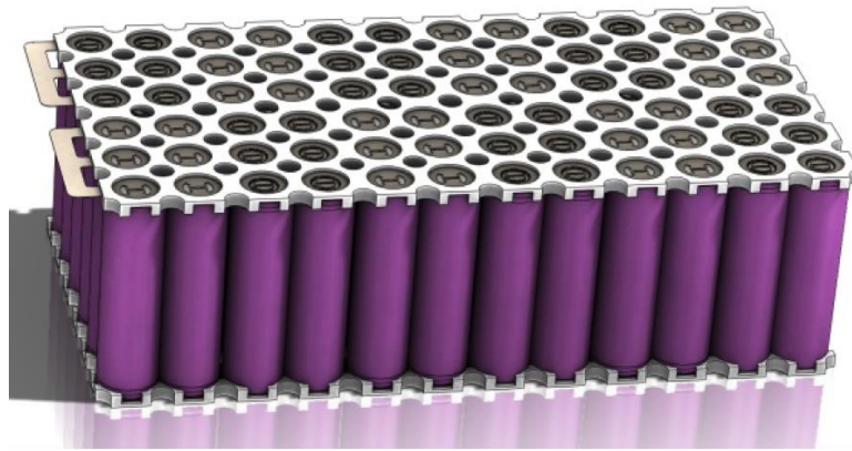
Figure 17: Existing technology, such as our design based on parallel strings Panasonic 18650 battery cells as illustrated, can be adapted to meet the unusual power requirements of PERISCOPE.
