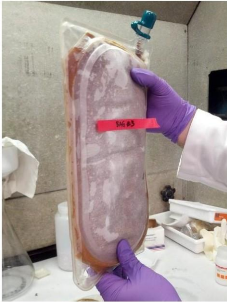
Figure 18a. XPack filled with fecal simulant and urine brine at start of experiment.
