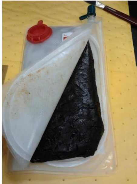
Figure 18b. XPack cut open to show solids material at the end of the experiment
