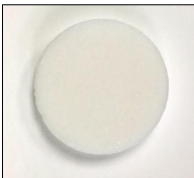
Figure 2.2-1. A rigid, round, potassium bromide sintered tile in the form of a thin white disk.
