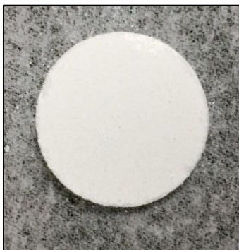
Figure 2.6-1. A sintered potassium bromide – yttrium oxide sample appearing as a white disk.
