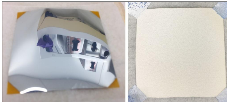
Figure 4.3.2-4. Silver-coated Kapton™-HN before and after coating with an airbrush using the methanol mixture. The silver-coated Kapton is highly reflective and after coating, is white and highly diffuse.
