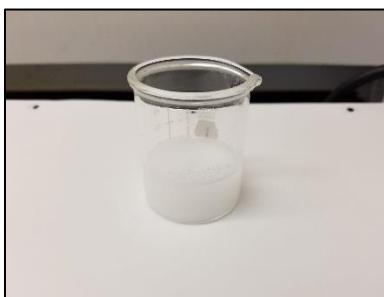
Figure 2.1.3-1. Barium fluoride sol-gel mixture used to determine if an alternative approach to sintering could be used to create a scattering layer.
