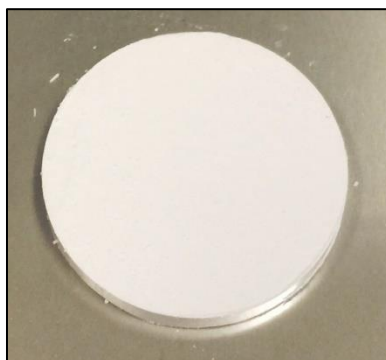
Figure 2.5-1. A sintered barium fluoride – hafnium oxide composite sample appearing as a white disk.
