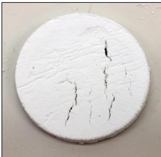
Figure 2.1.2-2. An example of a sintered barium fluoride sample produced with water content between 19% and 29%. The resulting tile has gaps in its surface, resembling cracks, where the material separated during sintering.
