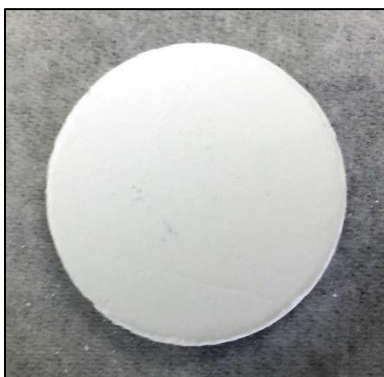
Figure 2.3-1. A rigid, round, hafnium oxide sintered tile appearing as a white disk.
