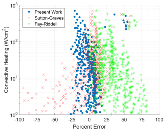
Figure 8. Updated convective heating correlation for Mars entry (blue dots) shows much smaller margins of uncertainty than historical correlations.
