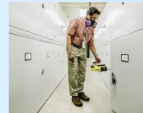
(Left) Roy Deza/GSFC is shown using a mercury analyzer to detect the levels of mercury vapor inside the cabinets during the installation and retrieval of MAC samples. Photo Credit: NASA/Chris Gunn
