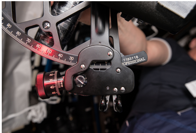
Figure 11. Sample Photo of Sextant Drum Scale During Sighting Session
