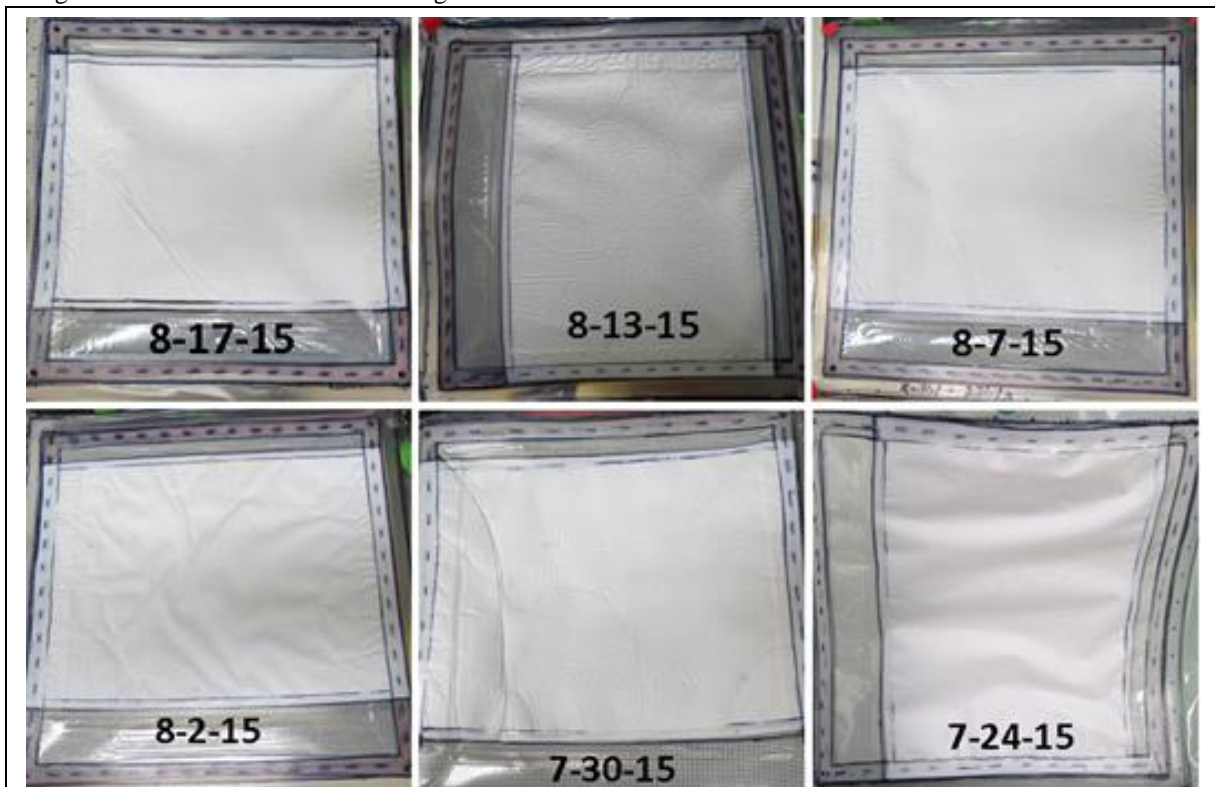
Figure 6. The membrane of the 6 Gen3 BEBs at the end of their runs. No evidence of membrane leakage is identified.
