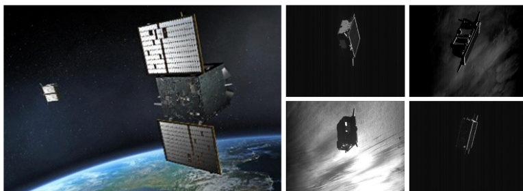
Figure 50.3 Graphical illustration of PRISMA technology demonstration mission (left). Images of the PRISMA's Tango spacecraft captured by the Mango close-range navigation camera during close-proximity operations at 10 m distance based on CPDGPS (right) [25]. Credits: OHB Sweden.
