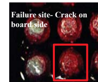
(a) Failure on board side
