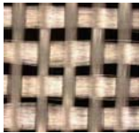
1080 Style Thickness: 63µm Nominal glass dia.: 5µm
