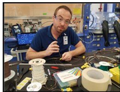
Figure 4. Wiring some thermocouples in the ACL.
