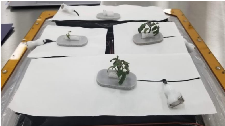
Figure 7. The rear and middle left plants suffered from salt burn caused by the wicks.
