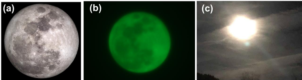
Figure 8. Full moon images taken from (a) Consolidated Lunar Atlas (NASA credit), (b) telescope setup by using the photon sieve, (c) iPhone 7. The results taken from the telescope with PS show the clear Moon focusing and filtering out near field objects such as clouds.
