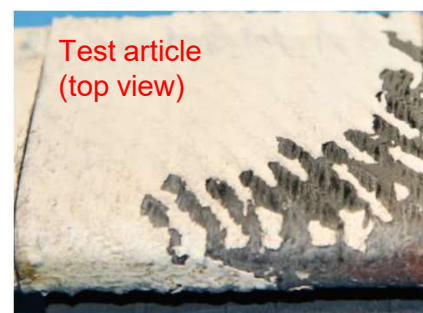
Spall of EB-PVD coating after 7 hours of 2700F cycles
