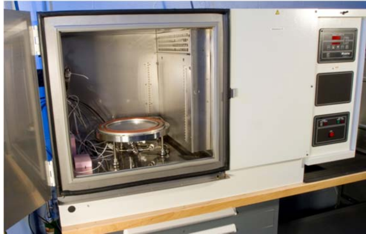
Figure 6. Seal leak test fixture installed in environmental control chamber. (Note: Top plate of test fixture not installed.)
