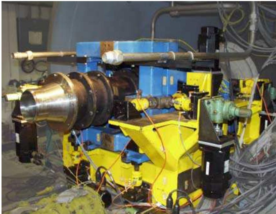
Figure 3: Thrust stand with ASME nozzle installed [3]
