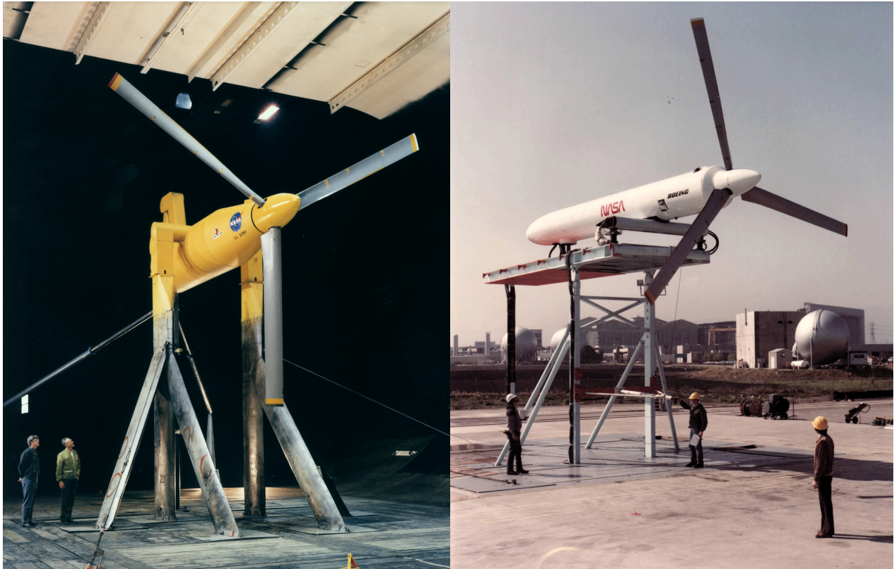
Figure 3. XV-15 rotor in the NFAC (left) and at the OARF (right).
