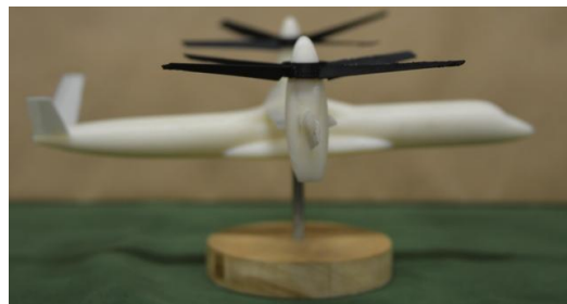
Figure 2B. The LCTR model with rotors in helicopter mode.
