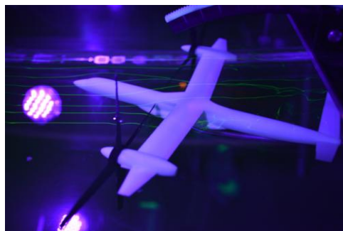
Figure 3A. Water channel results of the LCTR in airplane mode (isometric view).
