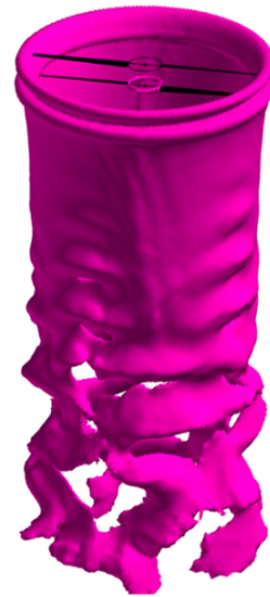
Fig. 7. Comparison of baseline and adaptive grid wake geometry ( \theta_U = \theta_L = 10^\circ ) for HC1 (Vorticity iso-surface) RotUNS steady calculations.
