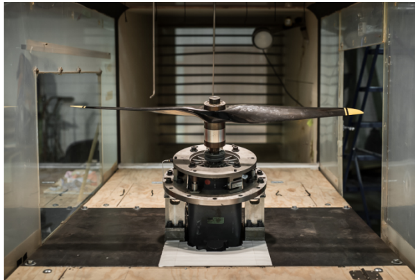
Figure 5. Single rotor at shaft angle -14 deg, looking downstream of the test section.
