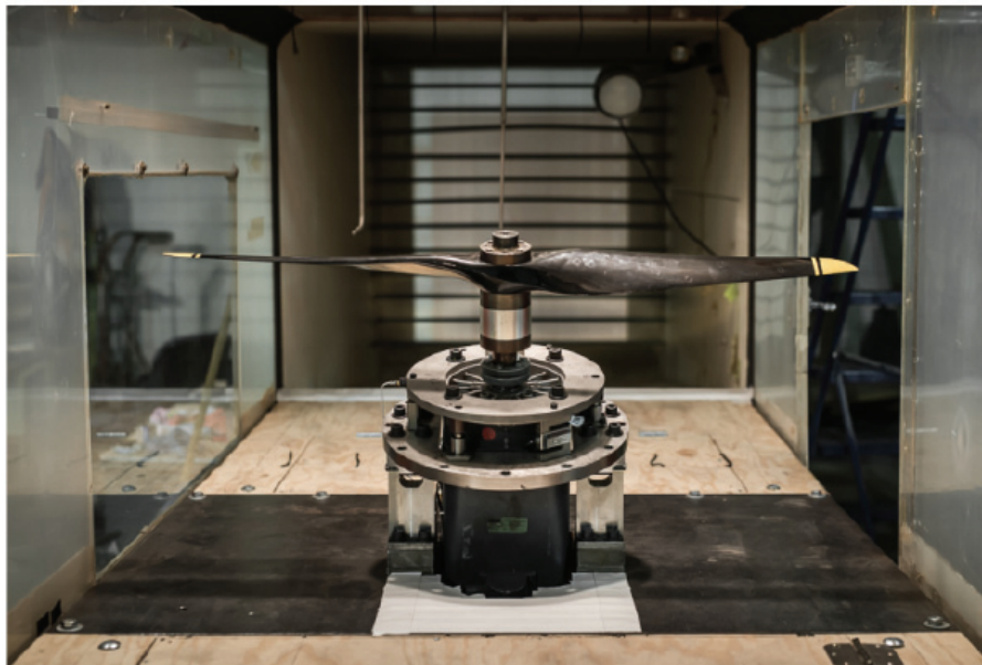
Figure 1. Single rotor at shaft angle of -14 degrees (ref. 1).
