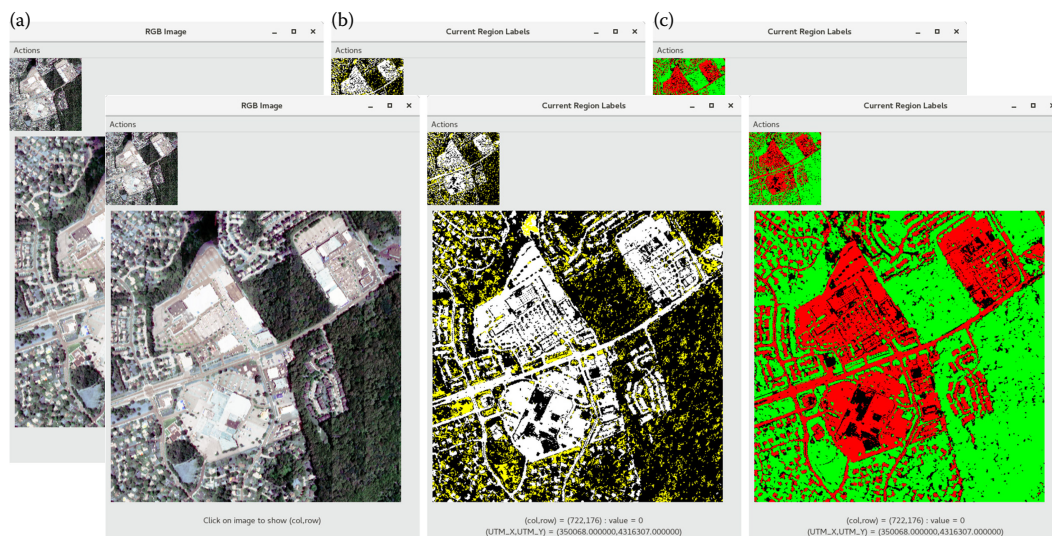
FIGURE 3.12 Example of using HSegLearn to generate a ground reference map of vegetation. (a) RGB image panel displaying a subsection of a hyperspectral image over a portion of downtown Bowie, MD. (b) HSegLearn Current Region Labels Panel after selecting some positive example region classes (vegetation, yellow) and some negative example region classes (nonvegetation, white). (c) HSegLearn Current Region Labels Panel: the positive example regions (vegetation, green) and negative regions (nonvegetation, red); region labeling by finding the coarsest levels in the HSeg segmentation hierarchy that do not conflict with the analyst labeling. These hyperspectral data were obtained by NASA Goddard’s LiDAR, Hyperspectral and Thermal (G-LiHT) Airborne Imager on June 28, 2012, at a nominal 1-m spatial resolution. The data set has 114 spectral bands over the spectral range of 418–918 nm.
