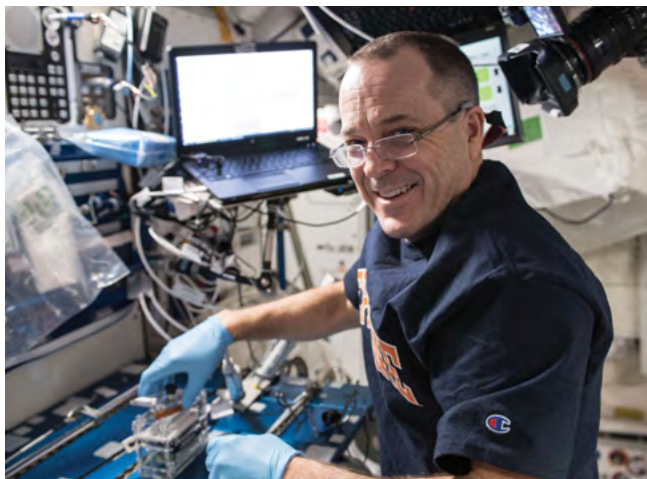
ISS crewmember Ricky Arnold, swabbing designated surfaces used to collect samples. He then used the Miniature Polymerase Chain Reaction (miniPCR) device to extract DNA from the samples (ISS056E097419).
