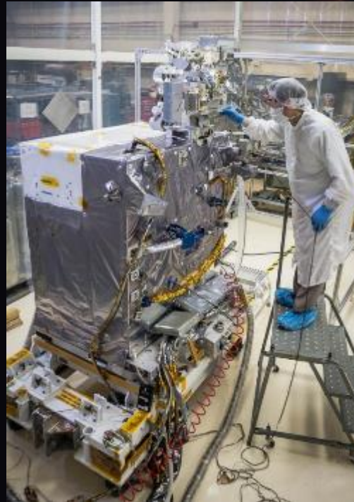
Robotic Refueling Mission (RRM) Phase 3 is a multi-phased International Space Station technology demonstration that is testing tools, technologies and techniques to refuel and repair satellites in orbit - especially satellites not designed to be serviced. Phase 3 demonstrates final tasks required to replenish cryogens in existing satellites not designed for servicing. Launched December 5, 2018
