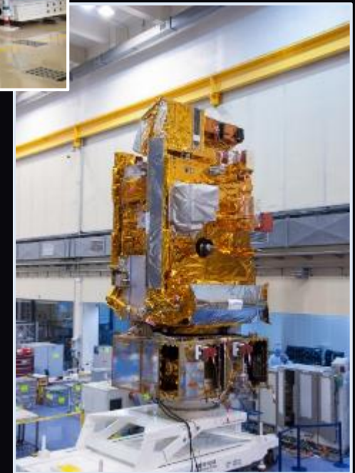
Meteorological Operational Satellite-C (MetOp-C) is the next (and last) in a series of three weather satellites from the ESA and EUMETSAT. Under Interagency agreements with NOAA, NASA (GSFC) is providing four POES heritage instruments AMSU-1, AMSU-2, AVHRR/3, and SEM. Launched: November 7, 2018
