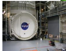
Chamber A: • 37m tall, 20m diameter, 12m door • LN2 shroud and GHe panels
