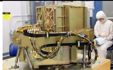
FGS: sense pointing to 1 millionth degree NIRISS: imagery & spectra of exoplanets
