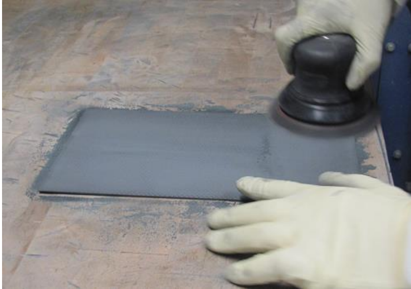
Figure 5. Manual ROS sanding of epoxy composite panel.
